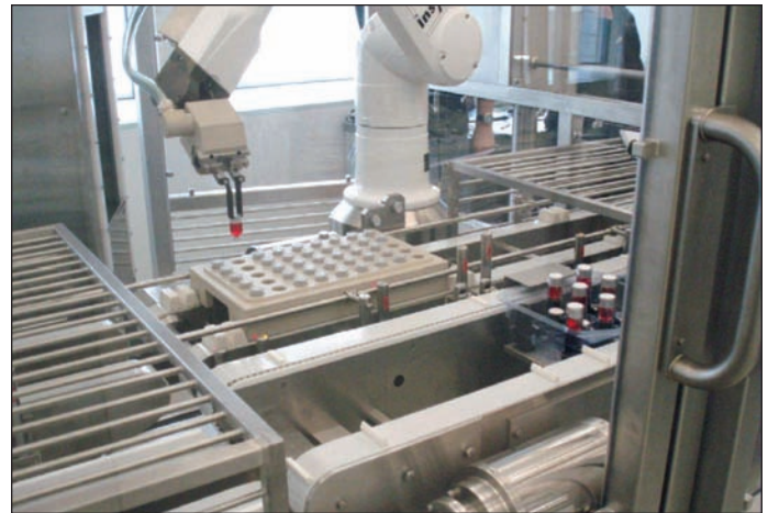
Robot picks a filled Vartridge.
