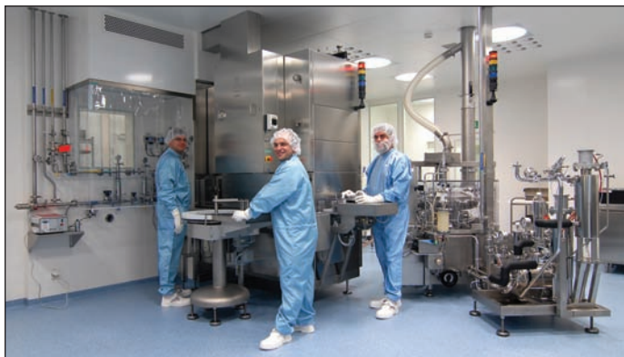
Vartridge filling and closing unit.
