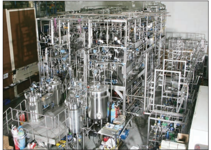
Fermenter super skid – assembled at vendor workshop prior to FAT.
