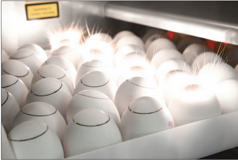
Eggs opened using an industrial scale laser process.
