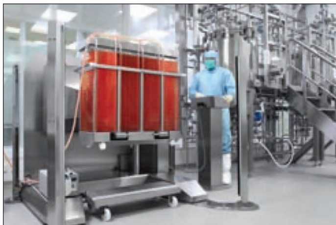
Fixed mixing inactivation and maturation vessels.
